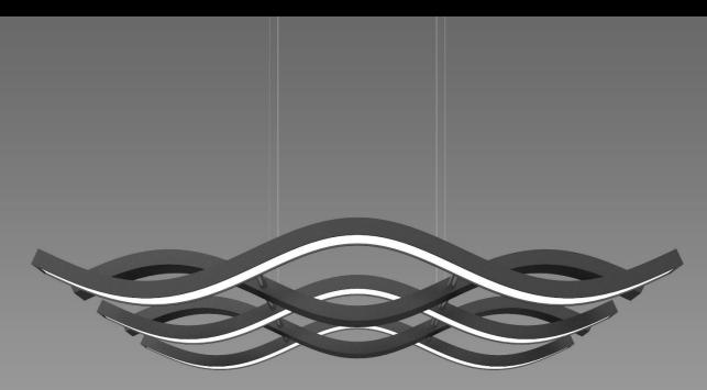
The five flowing profiles rise and fall side-by-side and combine three downlight and two uplight runs, creating the wave-like structure. Each of the five profiles act as a heatsink for the 120 LEDs, which are mounted along the runs. SINUS has a combined output of 6500lm and is suspended by Spectral's trademark cabling which doubles up as the power cable.
